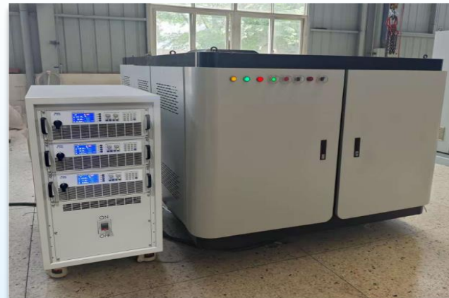
30 kW SOEC water electrolysis for hydrogen production
