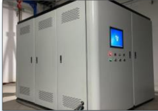
50 kW SOFC power generation system
